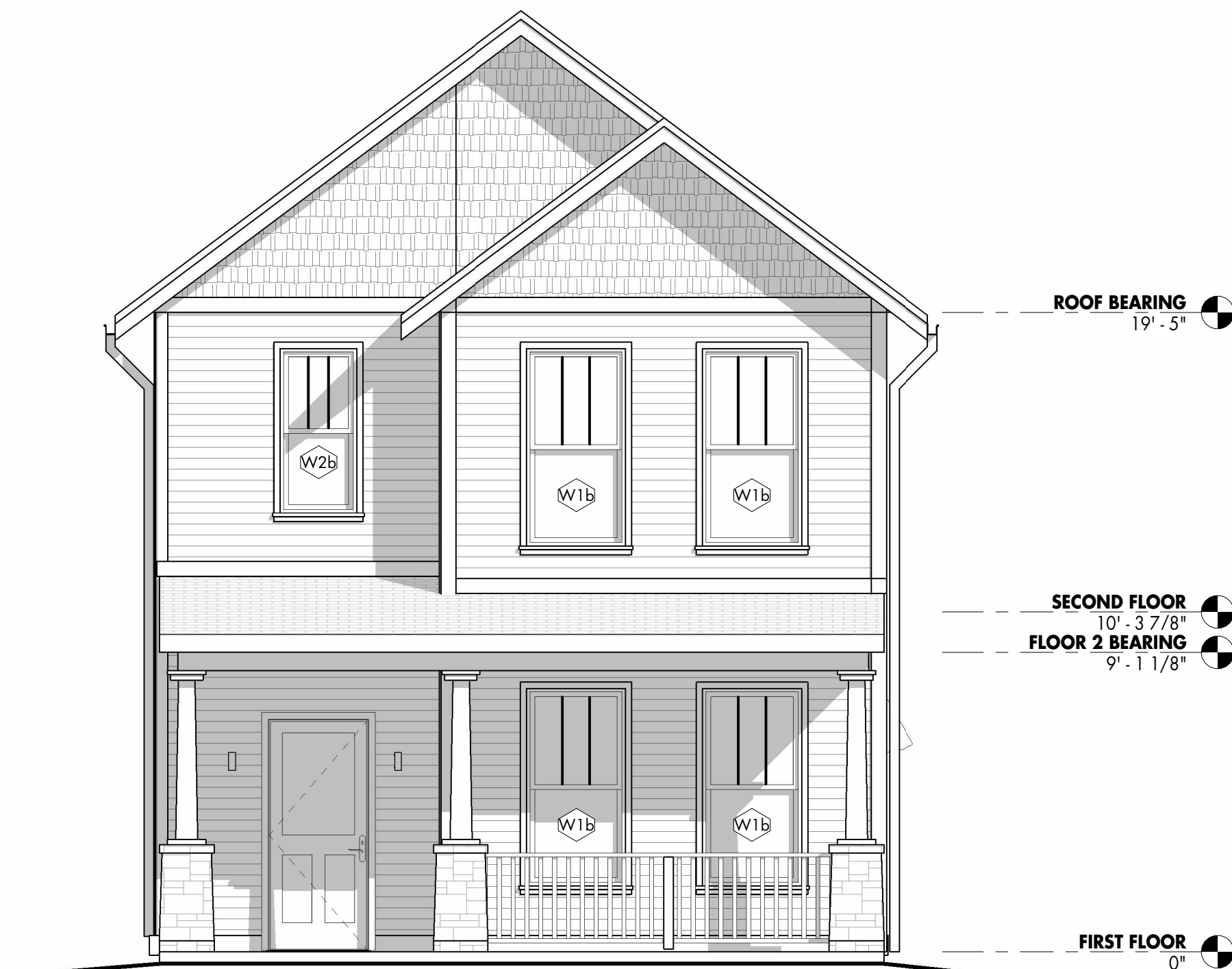
1 ELEVATION TYPE B - FRONT 1/4" = 1'-0"
