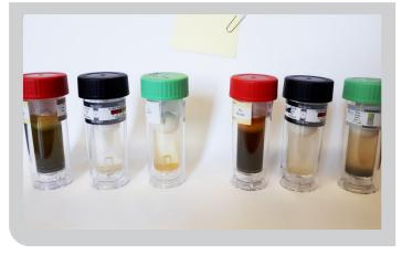
Using BART test kits, Environment Water was able to confirm the presence of aggressive IRB and aggressive slime-forming bacteria. Identification of the bacteria provided an understanding of the processes operating within the borehole, which highlighted the interactions taking place due to oxygenation of the borehole water column and mixing of water from different depths.
