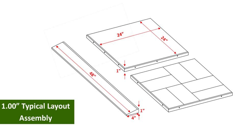
\* ALL MEASUREMENTS ARE NOMINAL AS RECYCLED RUBBER TILES ARE EXPECTED TO EXPAND AND CONTRACT WITH VARIATIONS IN TEMPERATURE AND UV EXPOSURE
