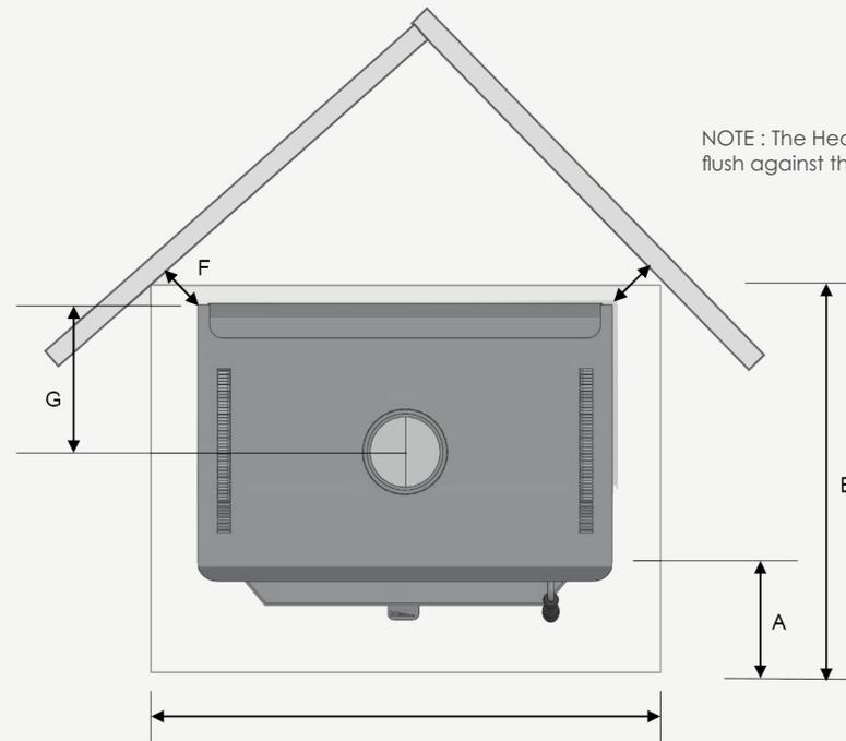
NOTE : The Hearth is not required to sit flush against the rear wall.
