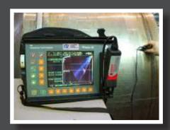
Hardness Testing – Qualified personnel and equipment for testing base materials, welds, and heat affected zones. Telebrineller Hardness and Ultrasonic Contact Impedance testing available.
