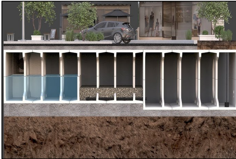
Figure 6: A multi-chamber treatment train designed by StormTrap, Inc.
