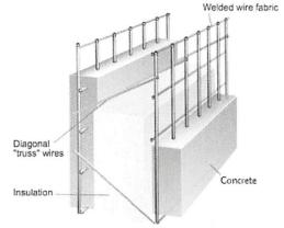
At Innovative Structural Solutions (Innstruct) we have developed a process that utilizes our Innstruct Structural Concrete Insulated Panel (SCIP) to create the Tilt-up Insulated Panel System (TIPS) as the primary structural and insulating member in conventional tilt construction.
