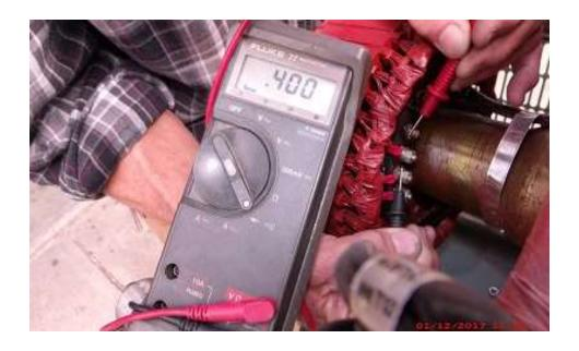
Put one of the leads of the ohm meter, with the meter set for the diode check scale, on the large screw on the diode pack. Then place the other lead on each one of the 3 smaller screws.
