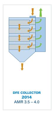
The graphic above shows an example of the Air-to-Media ratios for a typical weld fume application. The DFE features higher AMRs, smaller footprint, fewer filters, superior performance, and lowest cost of ownership!
